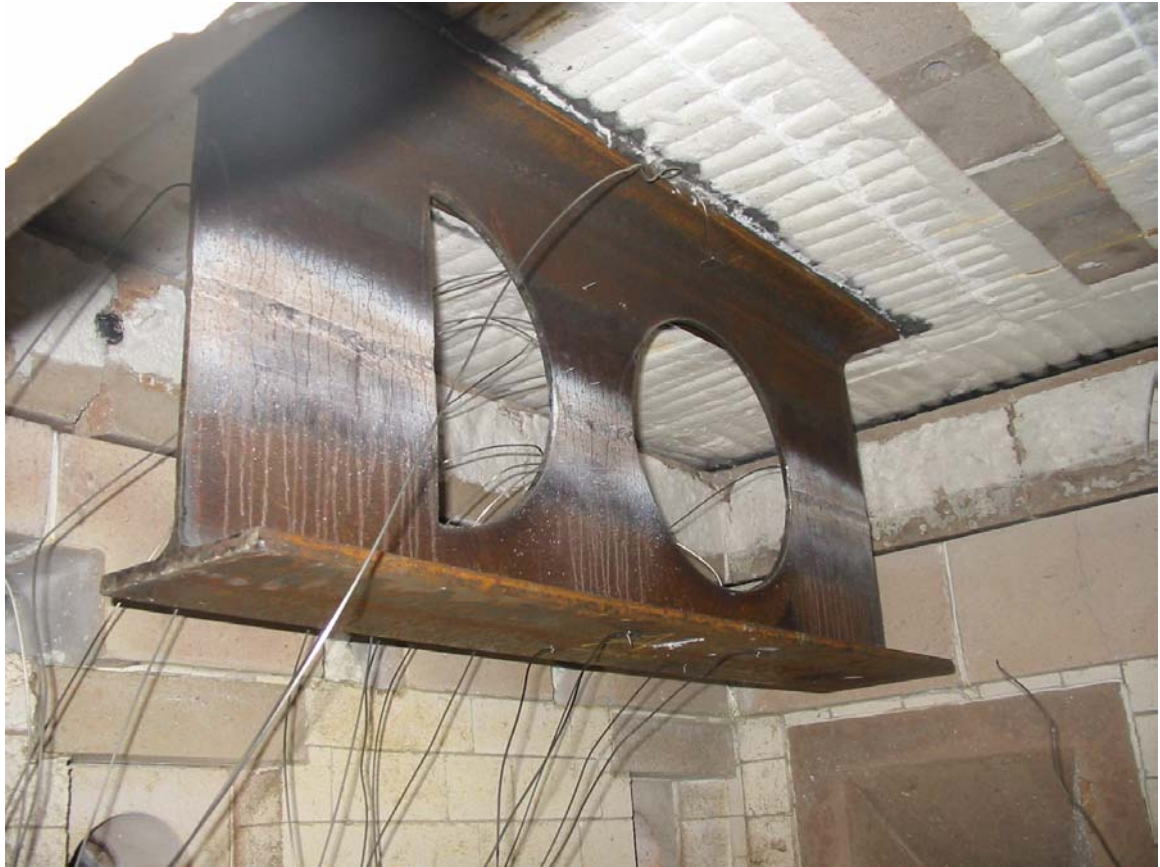
Figure 5 Photograph showing location of thermocouples on cellular beam.
